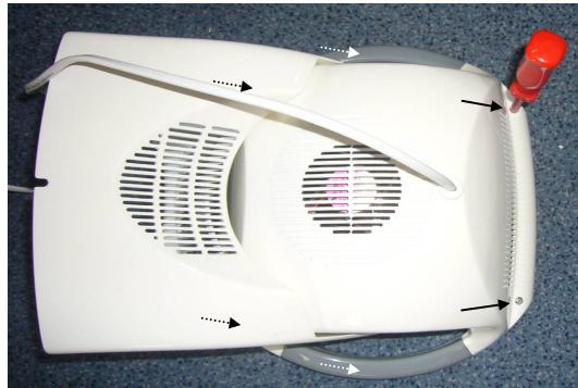
3. Place the body so that the front of the glass ceramic plate is lying on the flat surface.
